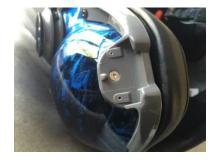
4) After drilling the right side mounting holes you can attach the right side of the chinstrap with the remaining (2) Phillip's head screws that were provided. When completed you should have (2) Phillip's head screws holding the left side chinstrap fastener to the helmet and also have (2) Phillips head screws holding the right side chinstrap fastener to the helmet. Therefore the only way to release or tighten the chinstrap is by using the quick release buckle with the Red Pull Tab.
